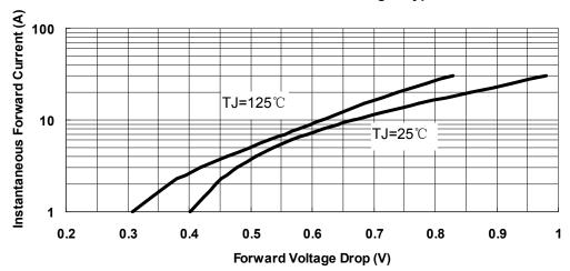
Fig.3-Typical Instantaneous Forward Voltage Characteristics
